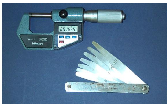
Figure G.1.2.3 A digital micrometre of resolution 0.001 mm and feeler gauges for sail cloth thickness measurement
